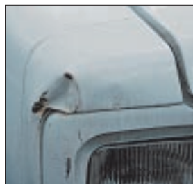
Any dent where primer or bare metal is exposed
