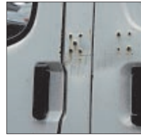
Damage where a fitting has been removed
