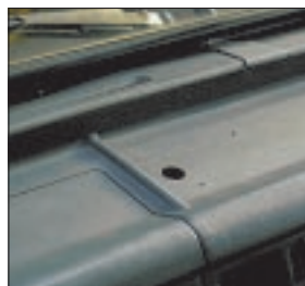
Untidy holes where after-market fitting has been removed
