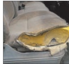
Damage to seat structure
