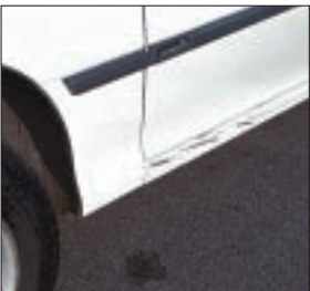
Heavy scratching below doors
