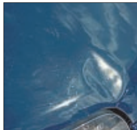
Any dent over 45mm in diameter
