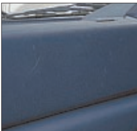
Light scratching due to normal wear
