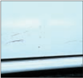
Isolated scratches up to 100mm in length
