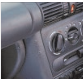
Neat holes where after-market fitting has been removed
